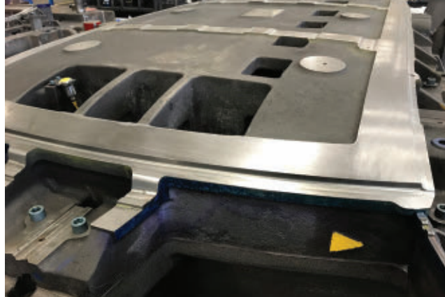
FIGURE 3. An example of automotive trim die used by the OEM supplier is shown; this die measures 177 × 95 × 54 in. and weighs 93,000 lbs.
