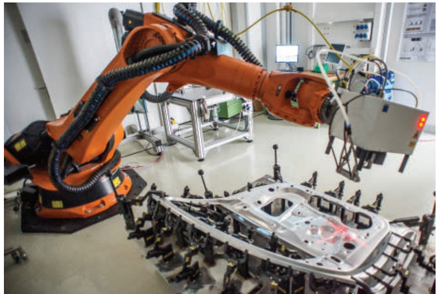
FIGURE 3. A typical installation for remote welding with high-power CW lasers is shown (IFSW, University of Stuttgart); in the future, similar facilities might also be used for highly productive micromaterials processing using kilowatt-class USP lasers.
