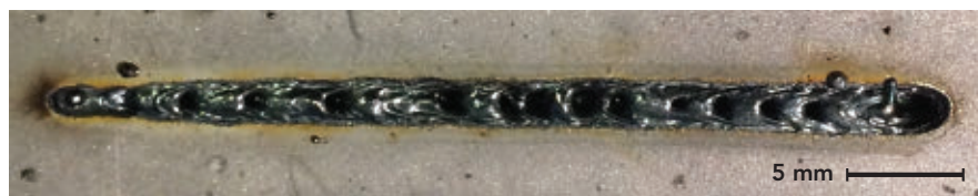
FIGURE 4. A result of zero gap lap welding of 1-mm-thick galvanized steel sheet at 3 kW output power and 1.5 m/min welding speed with a conventional single focused spot is shown.
