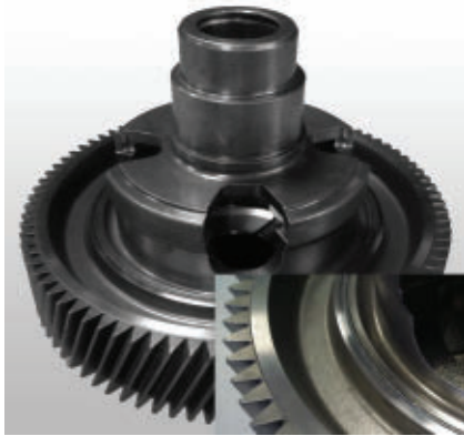
FIGURE 2. A laser-welded differential is shown.
