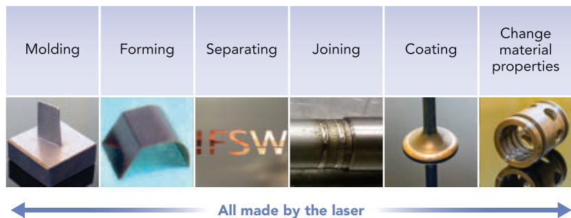
FIGURE 1. The laser can be used for materials processing applications that span the whole range of processes as defined by the German Industry Standard DIN 8580.
