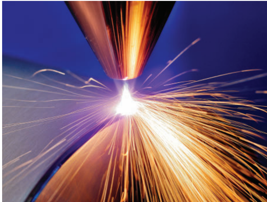
FIGURE 1. Laser material deposition is shown in action. (Copyright: Fraunhofer ILT, Aachen, Germany)
