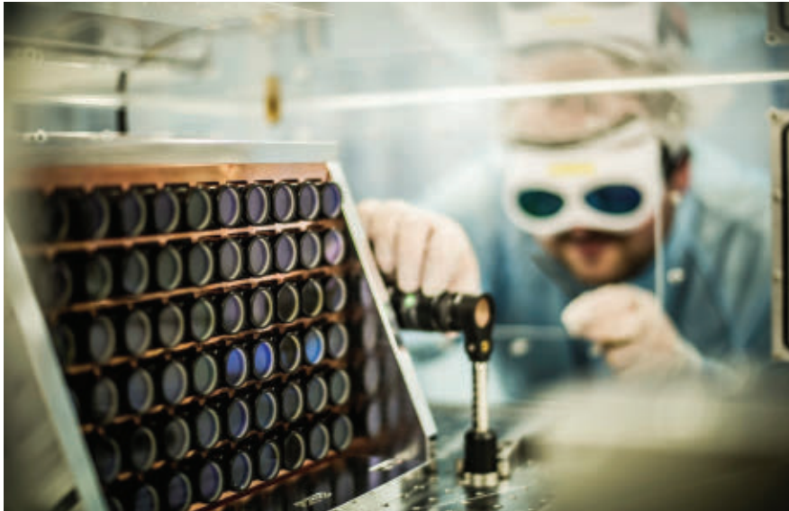
FIGURE 2. The heart of the multipass thin-disk laser amplifier developed at the Institut für Strahlwerkzeuge (IFSW), University of Stuttgart is an array of plane mirrors, which guides the laser beam with the ultrashort pulses to be amplified many times over the thin-disk laser crystal; 3,4 up to 2.5 kW of average output power with pulse durations of a few picoseconds have been demonstrated until now by this approach.
