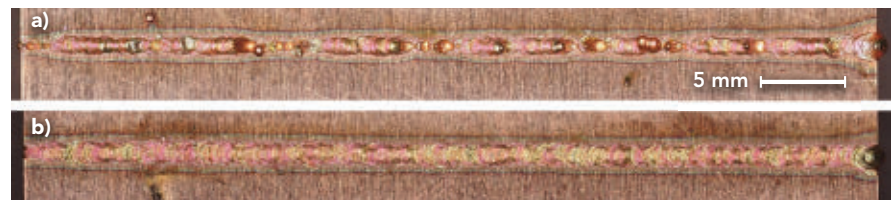
FIGURE 10. Welding bead appearance of pure copper using conventional single focusing spot (a) and beam mode control technology (b) are shown.
