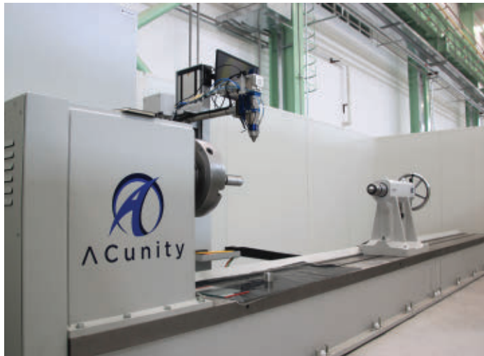
FIGURE 4. Hebei Jingye Additive Manufacturing Technology has received three EHLA systems; here, the 5-m-long compact system for components weighing up to three metric tons is shown. (Copyright: ACunity)
