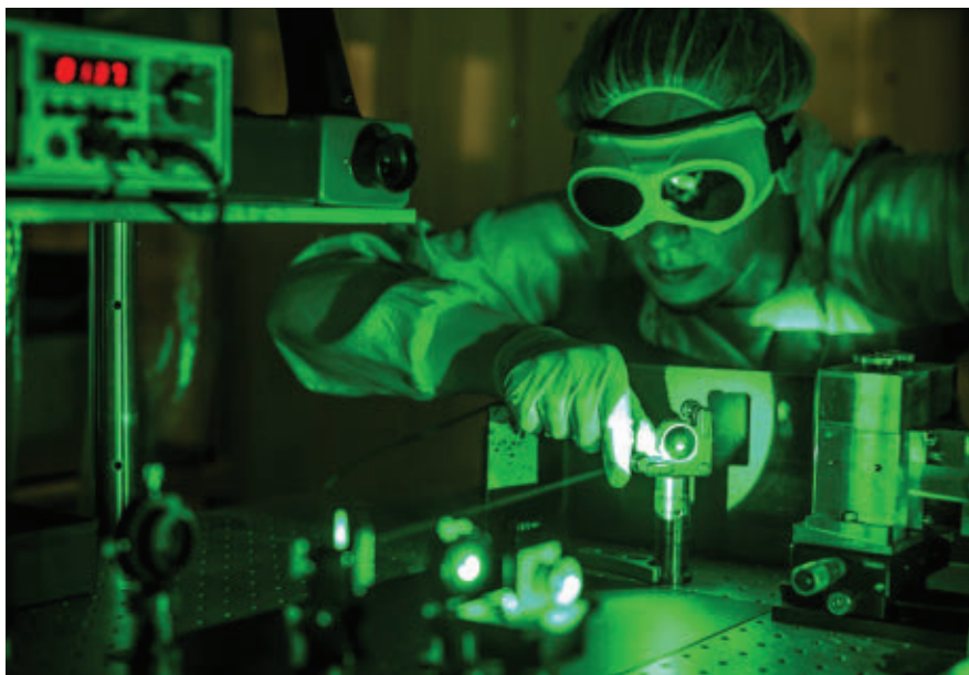
FIGURE 5. Intracavity frequency-doubling of a CW thin-disk laser is shown. 10
