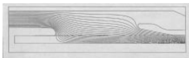
図4 絶縁筒の電界解析結果 Result of electric field calculation for designing splice body
