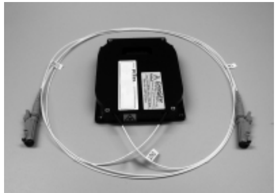
図6 Uncooled pump LD内蔵小型光ファイバアンプの外観図 Appearance of compact optical fiber amplifier with uncooled pump LD
