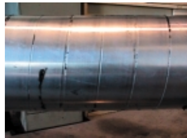
写真10 試験後の内圧補強層 Appearance of pressure reinforcements after laying test
