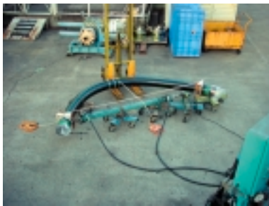
写真3 曲げ剛性測定状況 Measurement of flexural rigidity
