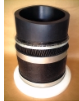
図5 軽量取水管の一般構造図及び外観 Structure and appearance of deep-sea water suction pipe of lightweight type
