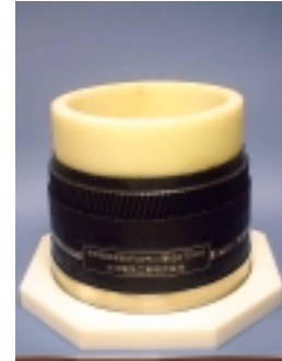
図6 PE-100適用取水管の外観 Appearance of deep-sea water suction pipe using PE-100
