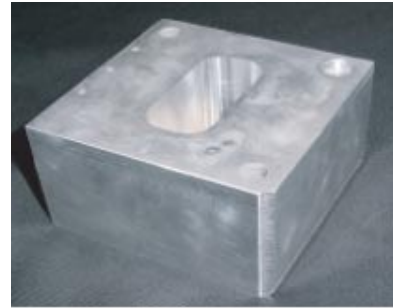
写真4-1 試作積層金型外観 Appearance of laminated EB mold.
