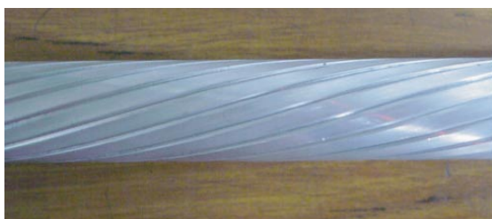
図2 CF-ACSR160 mm 2 の外観 Side view of CF-ACSR160 mm 2 .
