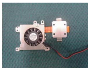
図5 世界最薄ヒートシンク Appearance of the world's thinnest heatsink.
