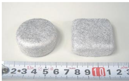
図4 深絞り試験サンプル Samples after deep drawability test.
