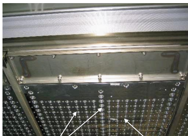
図2 ノズル付熱風噴出しパネル外観 Appearance of nozzle panel for hot-air discharge.
