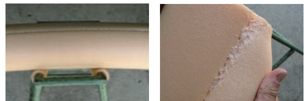
図4 断熱層の熱融着状態 Appearance of heat sealing line of thermal insulation sheet.
