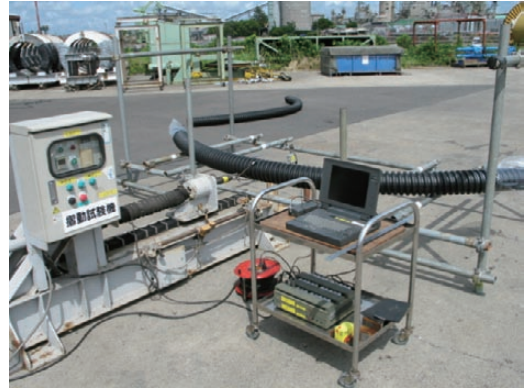
図8 曲げ剛性測定 (φ50) Measurement of flexural rigidity.
