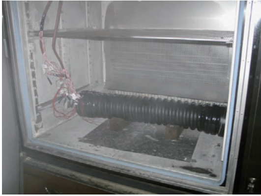
図10 断熱特性評価 (φ50) Freezing test.
