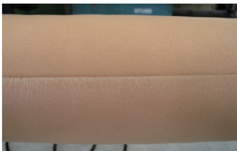
図7 曲げ試験後の断熱層 Appearance of thermal insulation layer after bending test.
