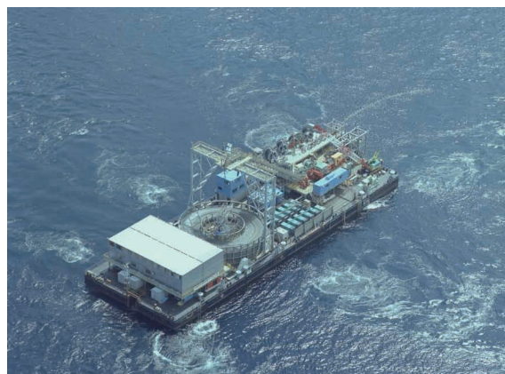
図8 純国産技術で構築されたDPS機能付布設船“天山” Cable-laying vessel with DPS function “Tenzan”, based on all-domestic technologies.
