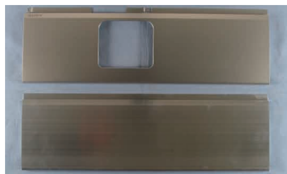
図7 アルミニウム押出型材 Aluminum extruded shape(Upper: As hairline treated. Lower: As extruded).
