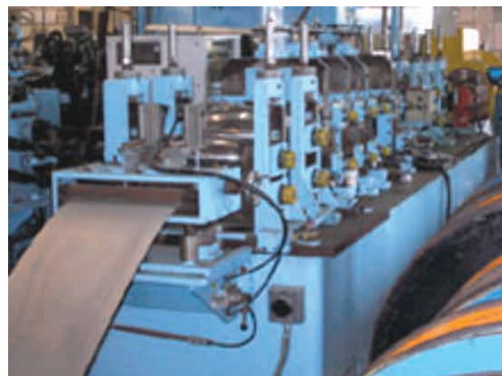
図2 連続自動造管機 Automated continuous manufacturing machine for thin-wall metal pipe.
