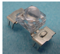
図3-1 LEDリード部とピアス端子の一体化 Integration of LED lead and pierce terminal.
