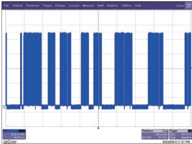
図12 光送信機のバースト光送信信号 Outgoing burst signal made from optical transmitter.
