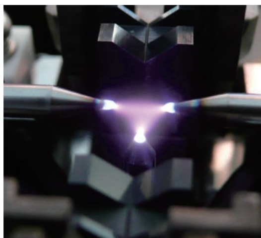
図8 3本電極間放電の写真 Appearance of 3-electrode arc discharge.
