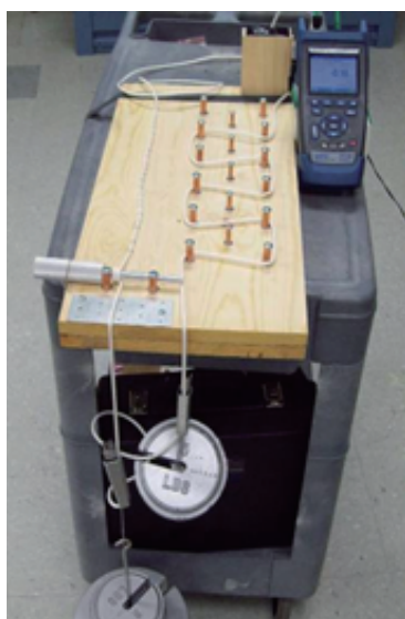
図2 集合住宅敷設模擬試験の装置例 Image of the MDU simulation apparatus for Verizon TPR 9424 testing.
