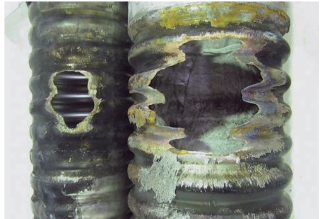
図4 AC10 kA 通電試料の断熱管損傷の様子 左側が断熱内管、右側が断熱外管 The damaged appearance of the cryostat pipe with AC 10 kA. The left is the inner pipe and the right is the outer pipe.
