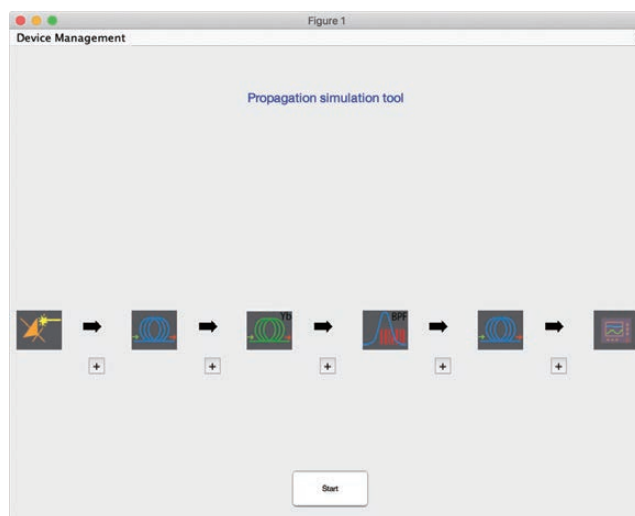
Figure 1 The main GUI window of PropSim with a few additional components compared to the initial state. From left to right the components are the followings: light source, a passive fiber, Ytterbium doped fiber, band-pass filter, passive optical fiber and diagnostic tool.
