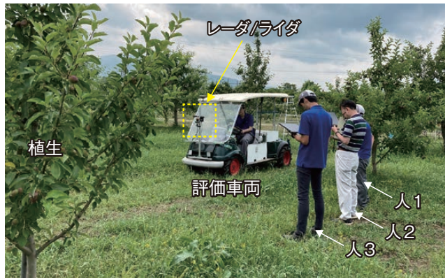
図6 レーダとライダーの測距性能の評価風景 Evaluation scene of distance measurement performance between Radar and LiDAR.
