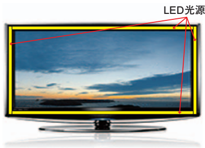
図4 光源の配置 Light source position.
