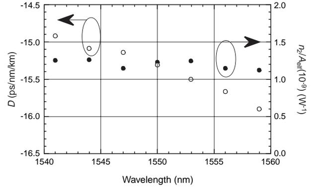
**Figure 8** Measured values of nonlinear coefficient  $n_2/A_{\text{eff}}$  (•) and chromatic dispersion  $D$  (o) for 830-m RDF
