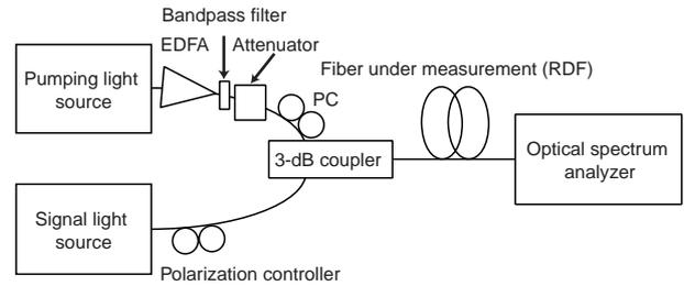
Figure 5 Setup for simultaneous measurement of nonlinear coefficient and chromatic dispersion
