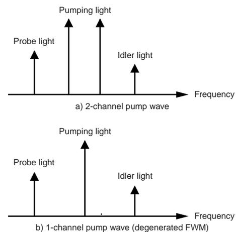
Figure 1 Schematic of four-wave mixing in the frequency domain
