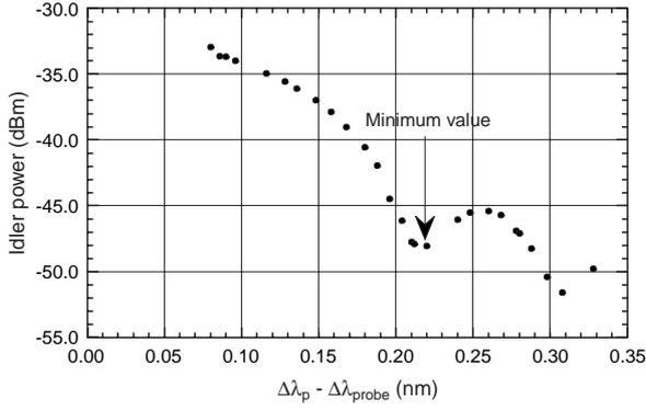
**Figure 7** Relationship of idler power to probe wavelength for a 10-km fiber with a pumping wavelength of 1553.0 nm
