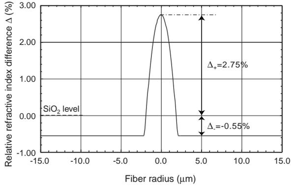
Figure 2 Refractive index profile of HNL-DSF
