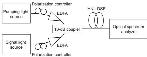
Figure 3 Setup for wavelength conversion experiment
