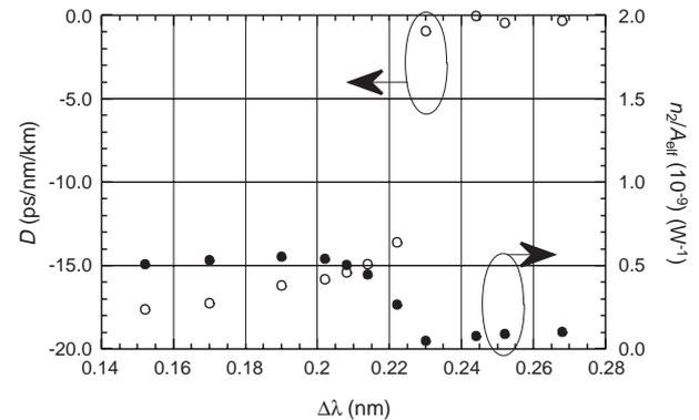
Figure 6 Measured values of nonlinear coefficient  $n_2/A_{\text{eff}}$  (●) and chromatic dispersion  $D$  (○) for 10-km fiber with a pumping wavelength of 1553.0 nm
