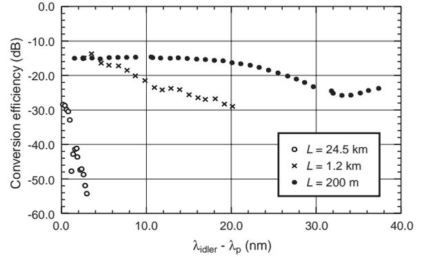
Figure 4 Measured values of conversion efficiency for fibers of selected lengths
