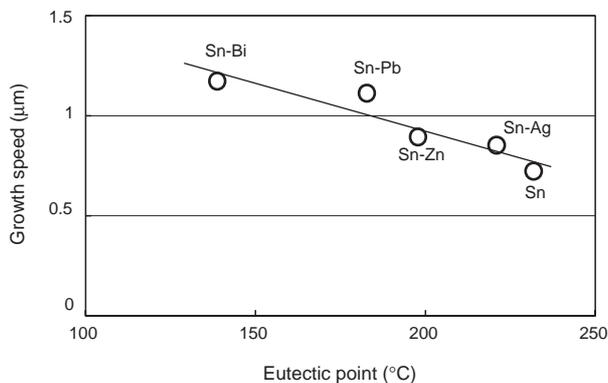
Figure 1 Relationship between eutectic point and intermetallic compound growth speed
