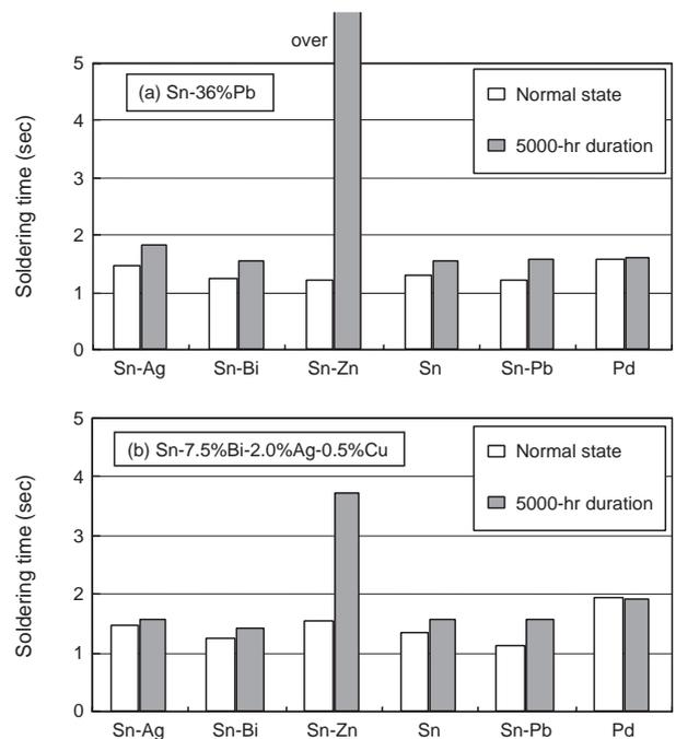
Figure 2 Wettability of Sn-Pb solder (a) and Pb-free solder (b)
