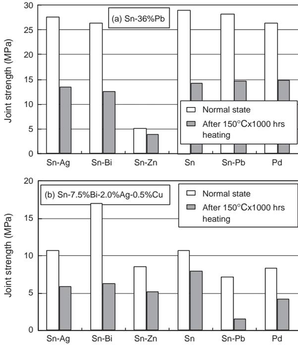
**Figure 3 Solder joint strength of Sn-Pb solder (a) and Pb-free solder (b)**
