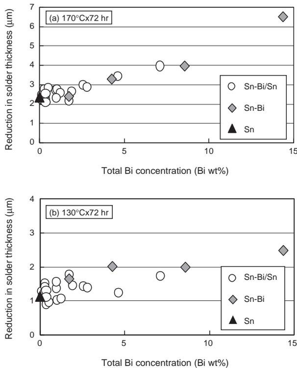
**Figure 4 Growth speed of intermetallic compound at 170°Cx72 hr (a) and 130°Cx72 hr (b)**
