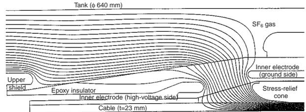
**Figure 3 Equi-potential line of electric field of dry type gas immersed termination**
