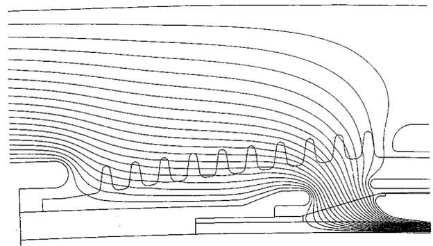
**Figure 4 Equi-potential line of electric field of dry type oil immersed termination**
