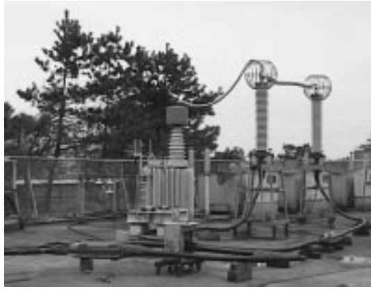
Photo 4 Test circuit for heating cycle test
