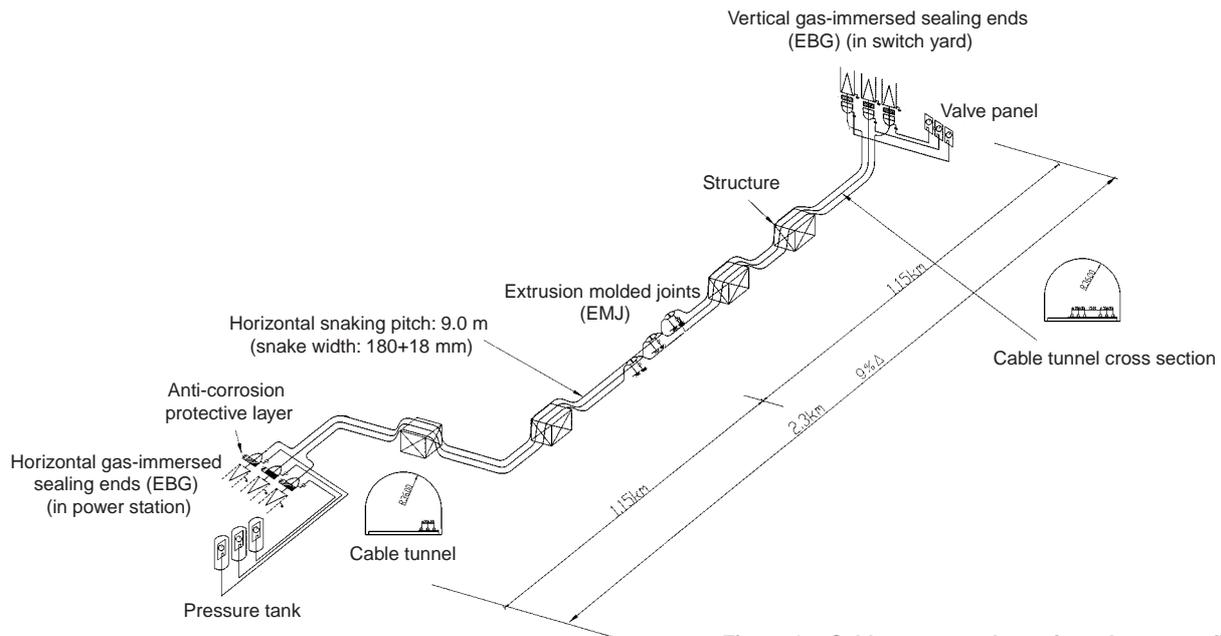
Figure 1 Cable system schematic and route profile
