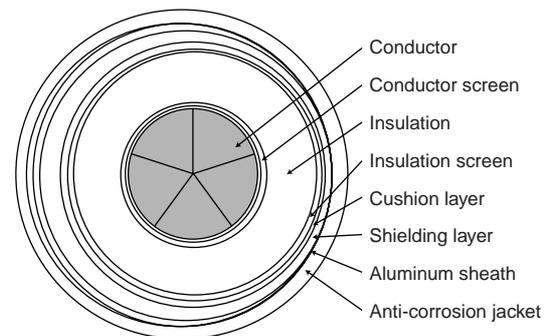
Figure 2 Cross-section of 500-kV XLPE cable (1 x 1000 mm<sup>2</sup> conductor)
