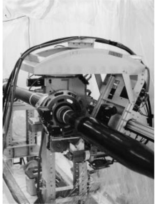
**Photo 7** System for photographic inspection using imaging plates
