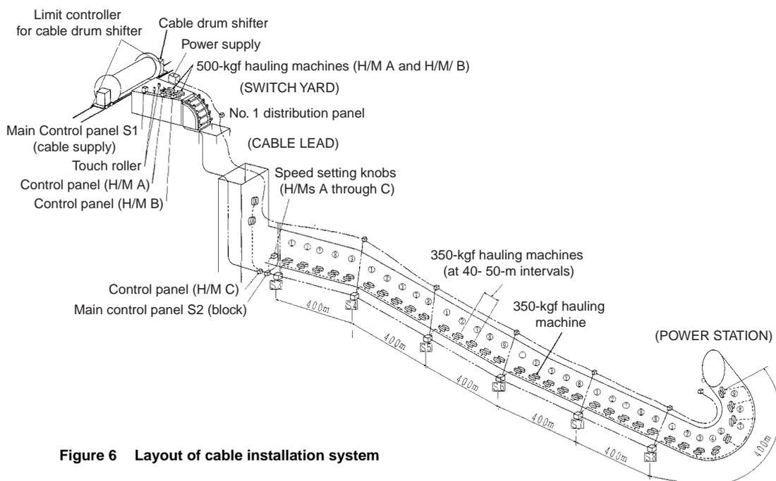
Figure 6 Layout of cable installation system
