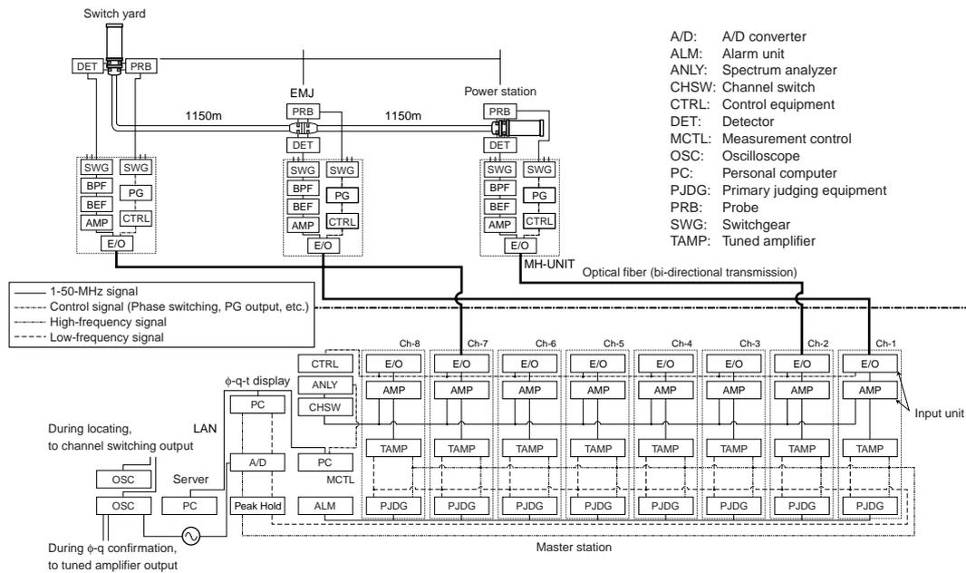
Figure 7 Block diagram of system for measurement of partial discharge
