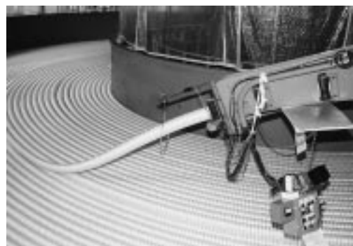
Photo 2 Storing the cable core into a large vessel for drying and oil impregnation
