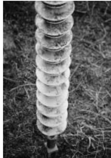
Photo 2 Composite insulator after application of power arc
