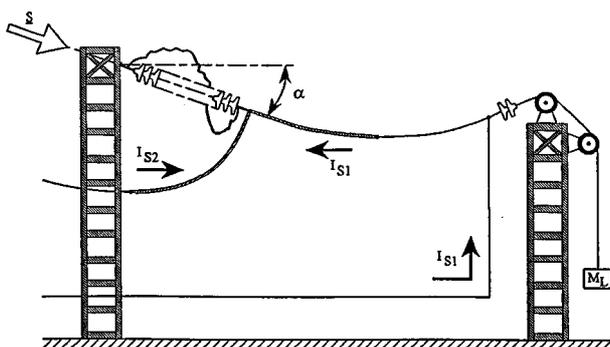
Figure 3 Setup for power arc test of composite insulator
