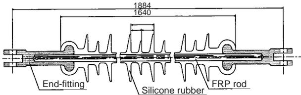
Figure 1 Structure of composite insulator
