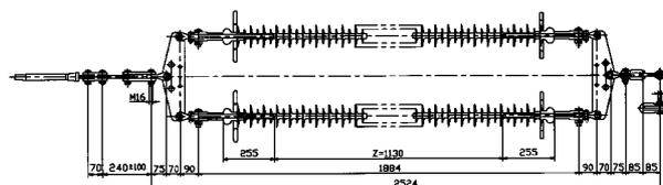
**Figure 2 Composite insulator string for tension tower**
