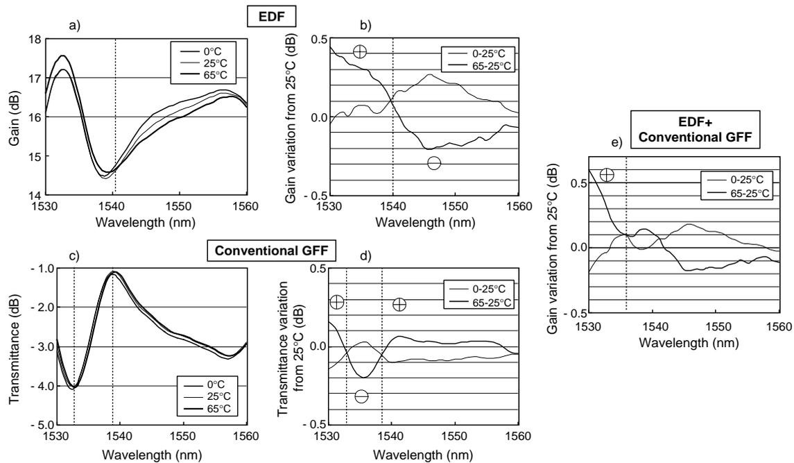
Figure 1 Temperature dependence of EDF and GFF
