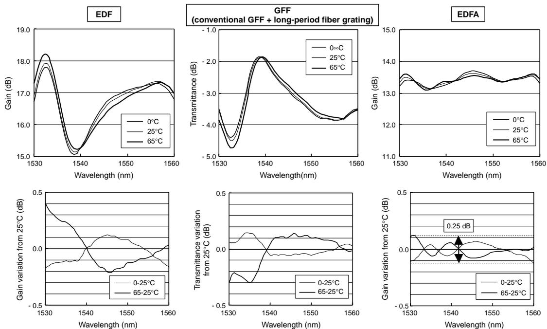
Figure 6 Characteristics of EDFA used in a prototype GFF with autonomous temperature stabilization of Erbium gain
