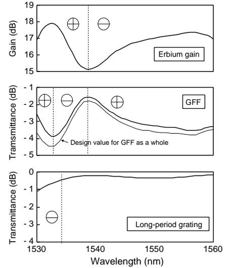
Figure 3 Characteristics of a GFF with long-period fiber grating
