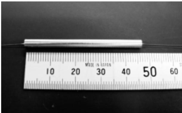
Figure 4 Photograph of long-period fiber grating module
