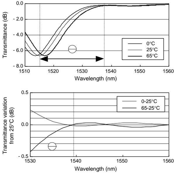
Figure 2 Temperature dependence of long-period fiber grating
