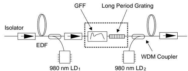
Figure 5 Configuration of EDFA with autonomous temperature stabilization
