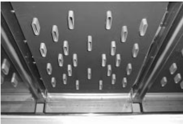
Photo 1 Panel heater used in the present system showing arrangement of nozzles
