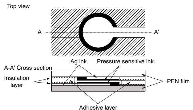
Figure 1 Schematic drawing of a flexible tactile sensor
