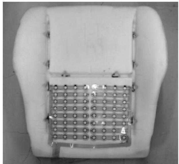
Photo 1 Installation of flexible tactile sensor mat
