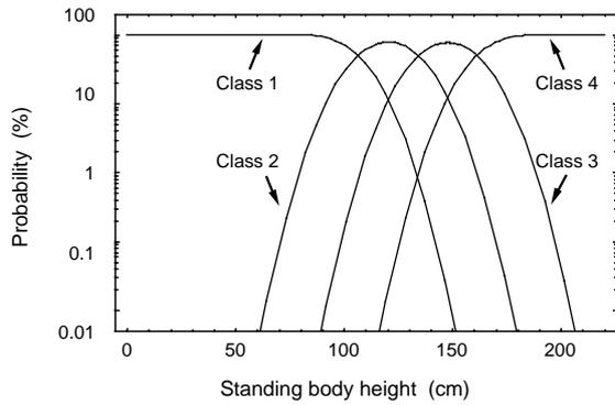
**Figure 8** Probability curves for classification calculated from experimental results for peak distance
