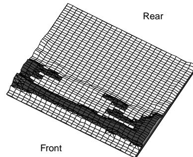
**Figure 10** Typical load distribution with child restraint seat on seat cushion
