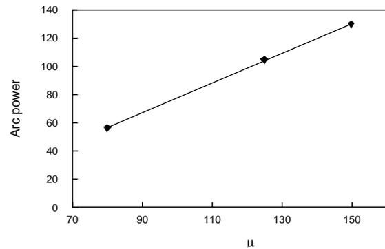
**Figure 6 Correlation between fiber diameter and arc power.**
