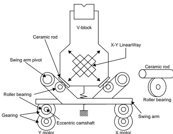
Figure 3 Aligning mechanism of the series S176.
