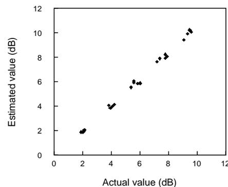
Figure 10 Accuracy of splice loss estimation for single-mode fiber.
