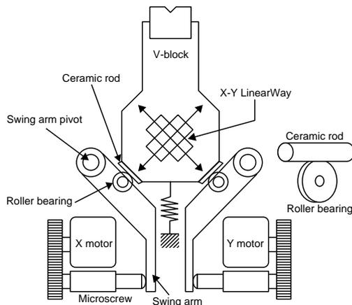
Figure 2 Aligning mechanism of the series S175.
