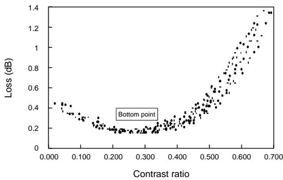
**Figure 4 Relationship between splice loss and contrast ratio for CS980 and single-mode fibers.**
