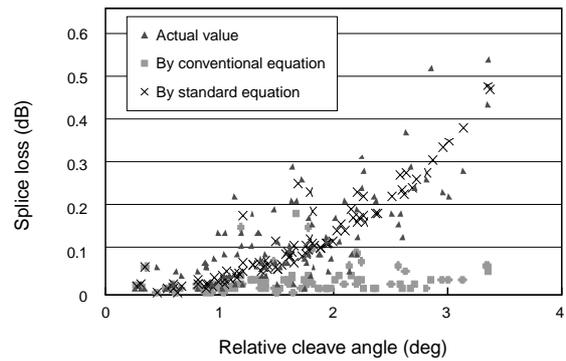
Figure 9 Comparison of accuracy of equations used to estimate splice loss.
