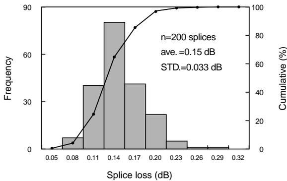
Figure 8 Histogram of splice loss for Corning CS980 and Furukawa single-mode fibers.
