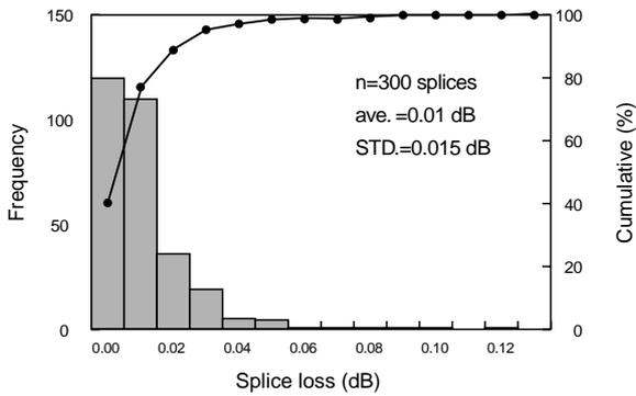
Figure 7 Histogram of splice loss for single-mode fibers.
