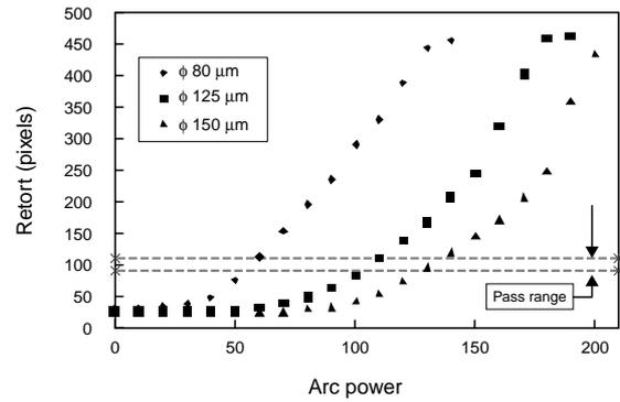
**Figure 5 Relationship between arc power and retort in fibers of different diameter.**
