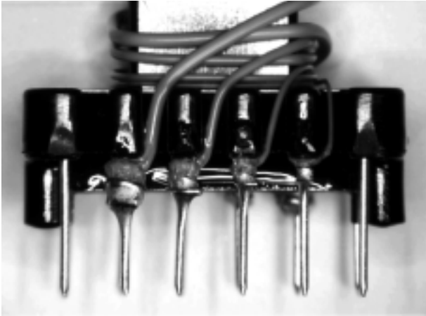
Photo 2 TEX-B wire after soldering.
