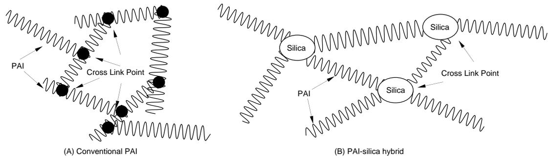
**Figure 2 Cross-linking model of conventional PAI and PAI-silica hybrid.**
