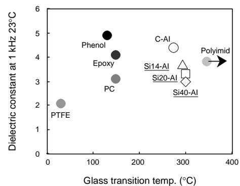
**Figure 1 Relationship between glass transition temperature and dielectric constant of various polymers.**
