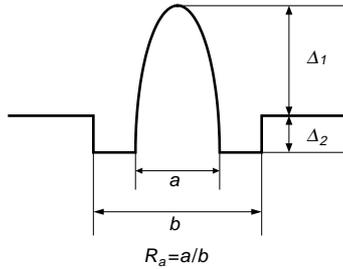
Figure 5 W-shaped refractive index profile detail.
