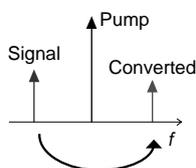
Figure 1 Conversion of a single wavelength by FWM.
