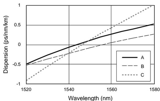
Figure 9 Dispersion characteristic of prototype fibers.
