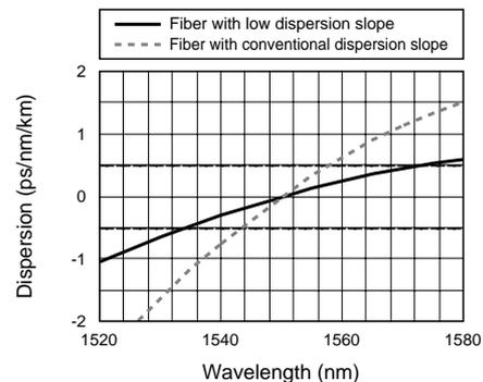
Figure 3 Wider bandwidth achieved by lower dispersion slope.
