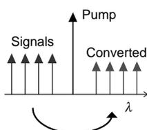
Figure 2 Conversion of multiple wavelengths by FWM.
