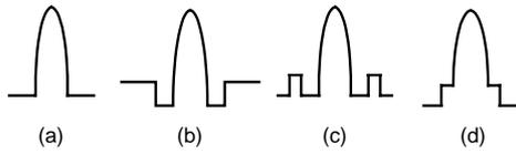
Figure 4 Representative refractive index profiles.
