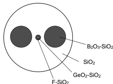
Figure 12 Structure of PANDA highly nonlinear fiber.
