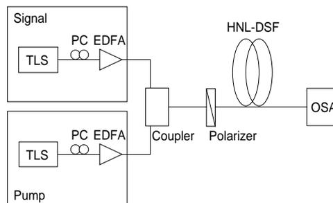
Figure 10 Set-up for wavelength conversion experiment.
