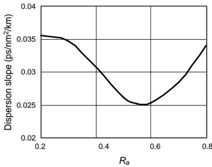
Figure 6  $R_a$ -dependence of dispersion slope.
