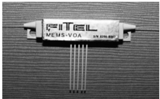
Photo 2 Appearance of MEMS-type VOA module.
