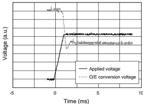
Figure 9 Switching time of insertion loss to 3-dB attenuation. (in matching oil for damping)
