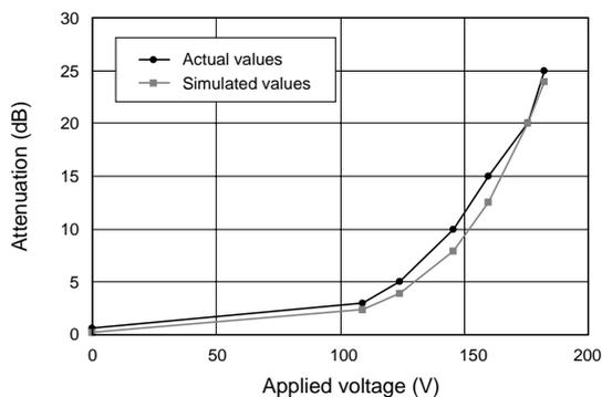
Figure 7 Voltage dependence of attenuation.
