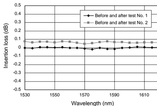
Figure 10 Change in insertion loss before and after vibration tests.
