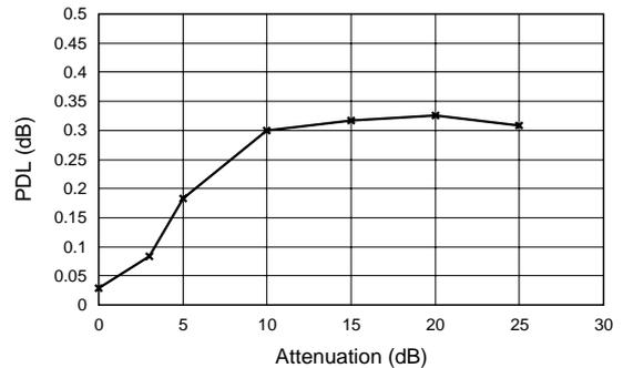
**Figure 5** Attenuation dependence of PDL.
