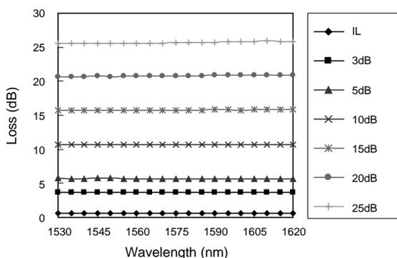
**Figure 4** Wavelength dependence of loss at selected values of attenuation.
