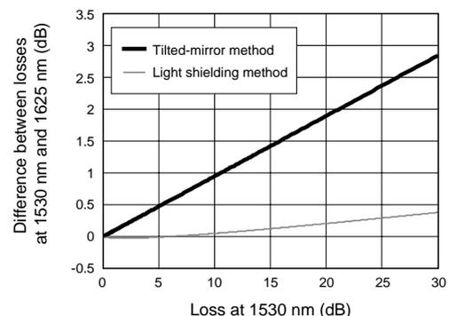
**Figure 1 Result of simulations of wavelength-dependent loss.**
