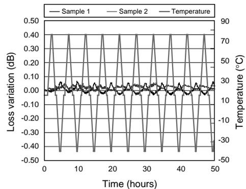
**Figure 6** Temperature dependence of insertion loss.
