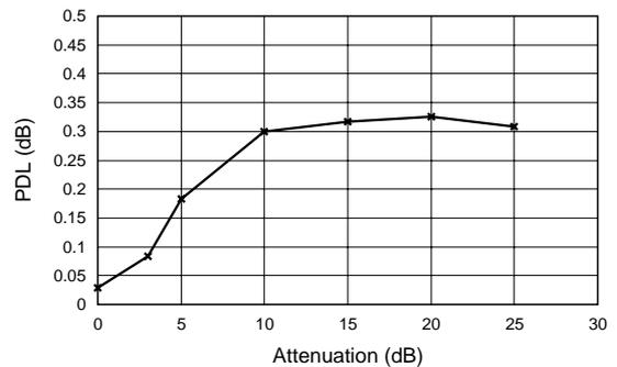
**Figure 5** Attenuation dependence of PDL.
