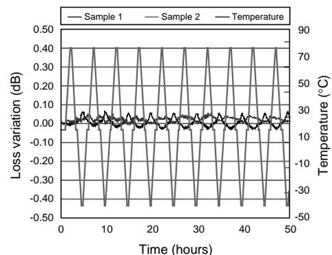
**Figure 6** Temperature dependence of insertion loss.
