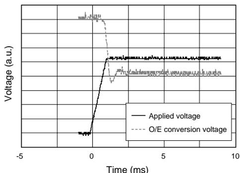
Figure 9 Switching time of insertion loss to 3-dB attenuation. (in matching oil for damping)
