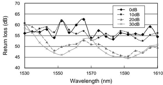
**Figure 3** Wavelength dependence of return loss at several values of attenuation by shutter. (at incidence port)
