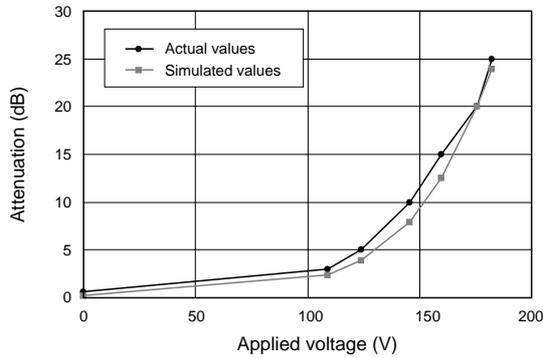
Figure 7 Voltage dependence of attenuation.
