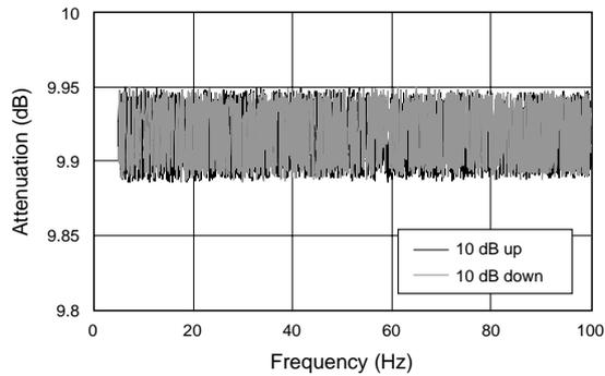
**Figure 12** Change in attenuation near 10 dB when acceleration and vibration added in Y direction.
