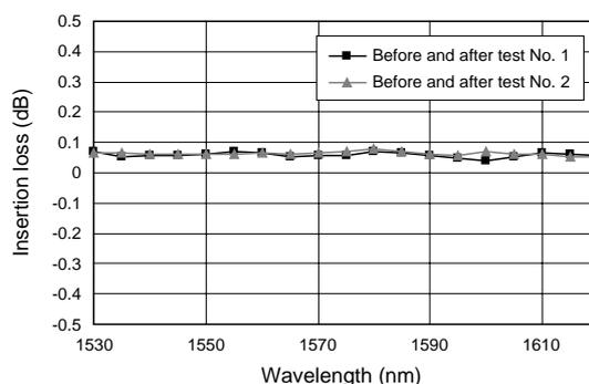
Figure 11 Change in insertion loss before and after impact tests.
