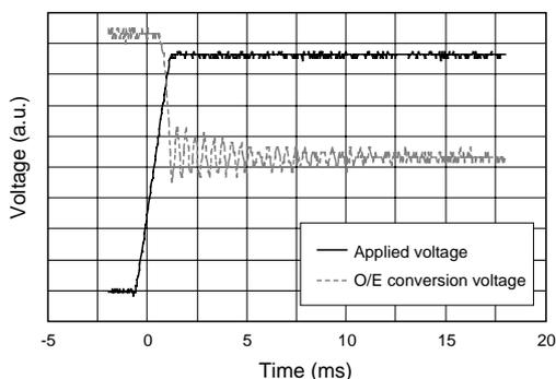
Figure 8 Switching time of insertion loss to 3-dB attenuation. (in air)
