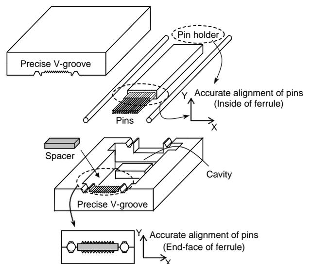
Figure 9 Structure of precise metal mold.
