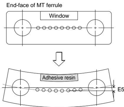
Figure 5 Bend by shrinking of adhesive resin.
