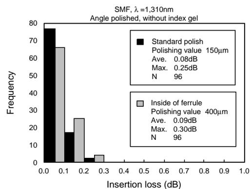
Figure 16 Insertion loss of low-loss MPO24 connector.
