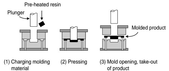
Figure 13 Transfer molding process.
