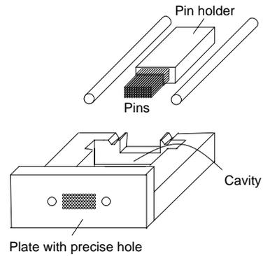
Figure 12 Super high-density ferrule metal mold.
