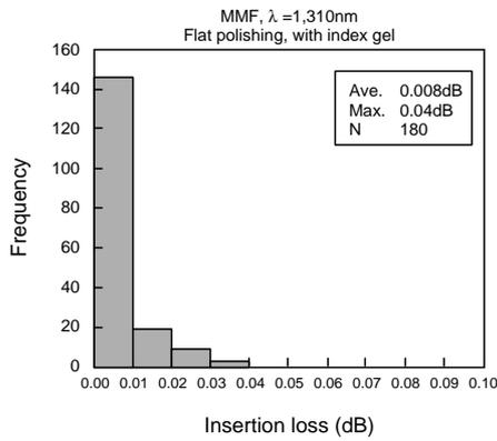
**Figure 18** Insertion loss of super high-density 60-fiber connector.
