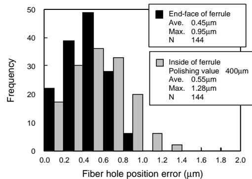
Figure 15 Fiber hole position error of low-loss MT24 ferrule.
