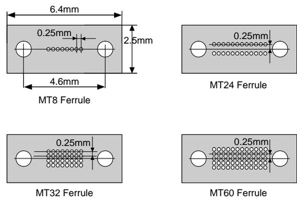
Figure 1 End-face of MT ferrules.
