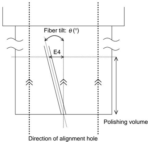
Figure 4 Fiber hole tilt.
