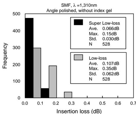
Figure 14 Insertion loss of super low-loss MPO8 connector.
