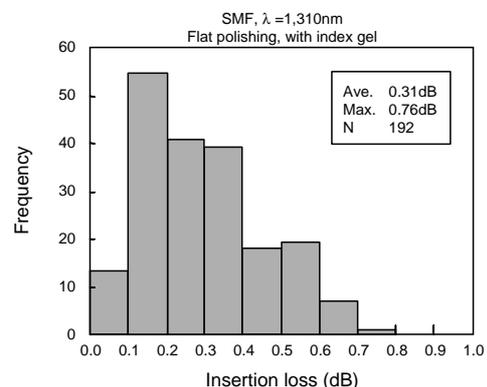
Figure 17 Insertion loss of super high-density 32-fiber connector.
