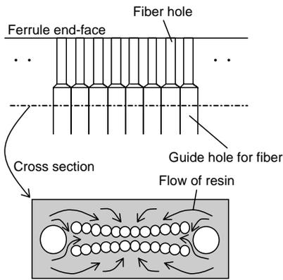
Figure 10 Structure of conventional pins.
