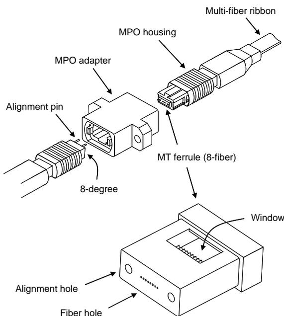
Figure 2 MPO connector structure.
