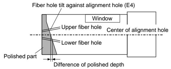
Figure 7 Fiber hole tilt of 2D-MT ferrule.
