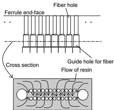
Figure 11 Structure of improved pins.
