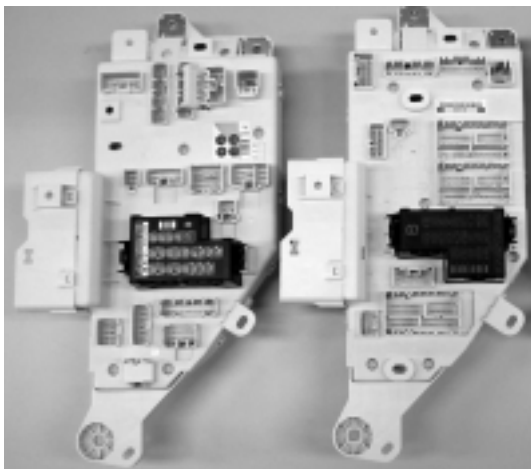
Figure 1 Appearance of J/Bs before (left) and after (right) minor model change.
