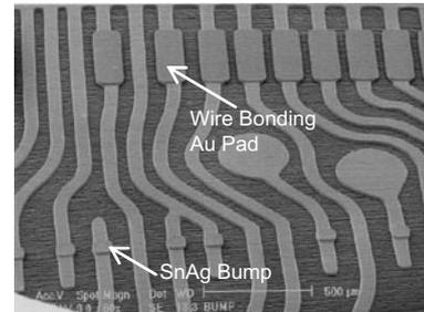
Figure 15 SEM image of bump side of the interposer shown in Figure 14.
