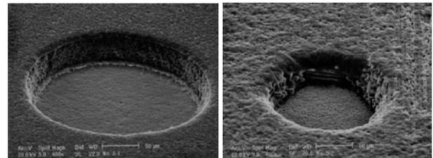
a) 40 μm-thick polyimide      b) 50 μm-thick glass epoxy
