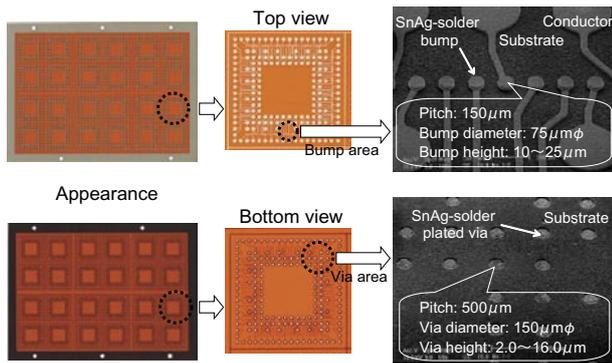
**Figure 1** Appearance of interposer using 40 μm-thick polyimide substrate.
