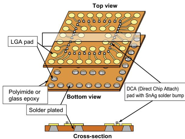
**Figure 2** Illustrative drawing of interposer shown in Figure 1.
