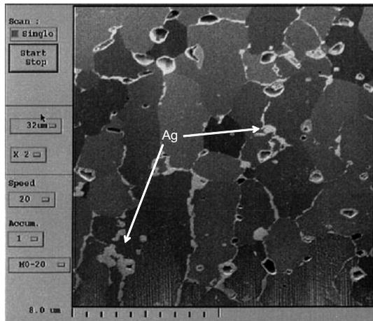
Figure 8 FIB-SIM image of SnAg-solder plating.
