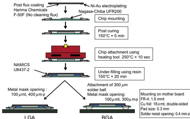
Figure 9 Sample preparation process for reliability evaluation.
