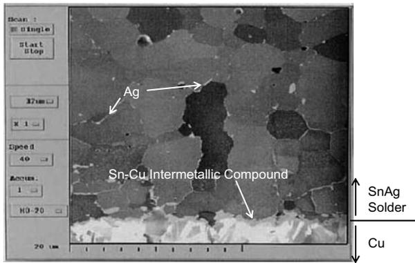
Figure 7 FIB-SIM image of the interface between Cu and SnAg-solder plating.
