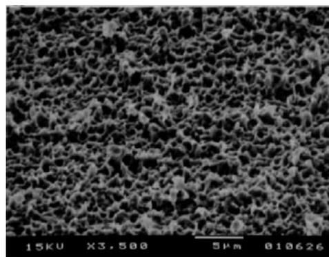
Figure 6 Cu foil surface after roughening treatment.
