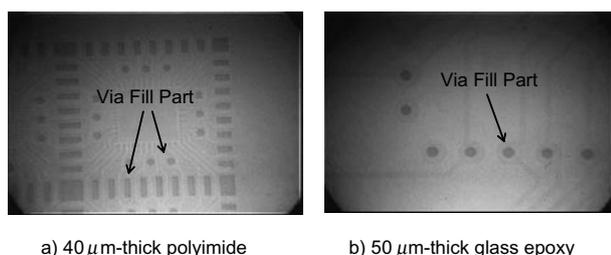
Figure 5 Soft X-ray images of via-filling.
