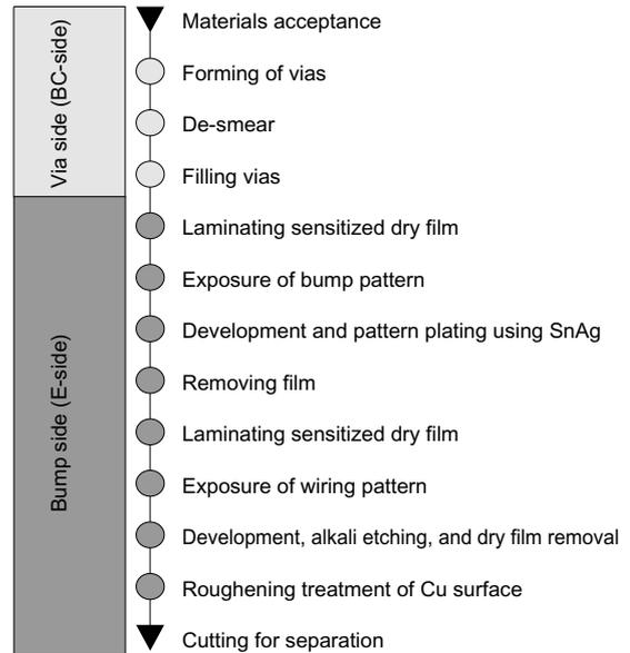
**Figure 3** Manufacturing process.
