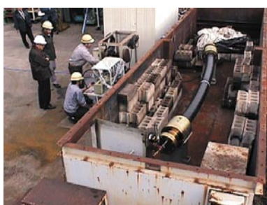
Photo 1 Burst pressure test.
