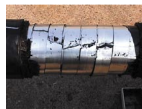
Photo 2 Burst point due to internal-pressure test.
