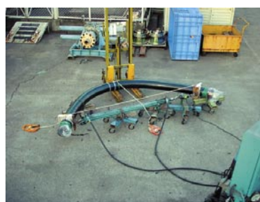
Photo 3 Flexural rigidity measurement.
