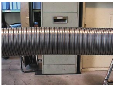
Photo 11 Appearance of interlocked conduit after laying test.
