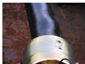
Photo 2 Burst point due to internal-pressure test.
