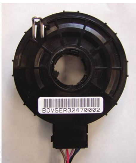
Photo 6 Appearance of steering torque and angle sensor.
