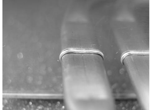
Figure 3 Photograph of stacked fin heatsink with flattened heatpipe.
