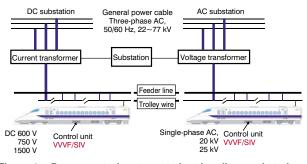
Figure 1 Power control system at electric railway substations in Japan.
