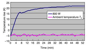
Figure 6 Low-temperature start-up characteristics of HP-VAH.
