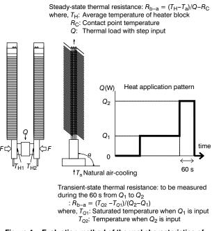
Figure 4 Evaluation method of thermal characteristics of HP-VAH.
