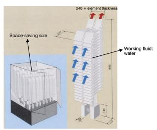
Figure 3 Cooling mechanism for HP-VAH.
