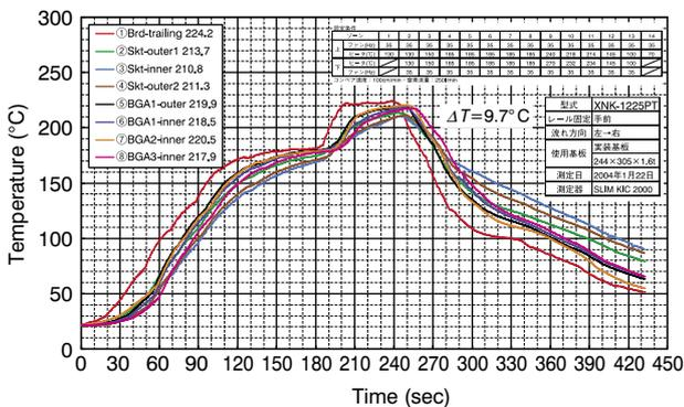
Figure 4 Typical temperature profile for test board.
