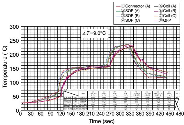
a) Previous XNK-945 system with conveyer speed of 80 cm/min
