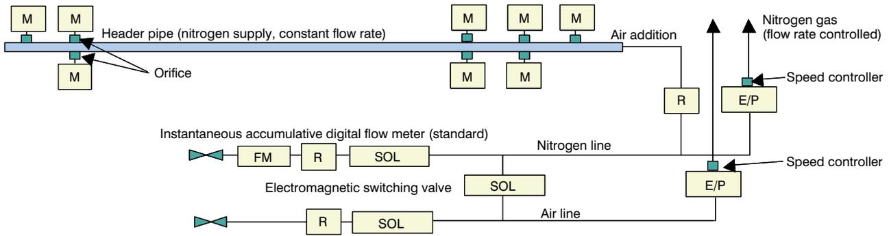
Figure 9 Nitrogen supply method.
