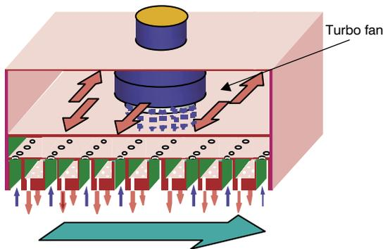
Figure 3 Convection heating engine.
