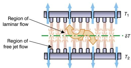
Figure 5 Principle of reducing temperature interference between top and bottom nozzles.
