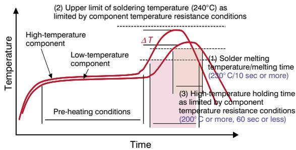
**Figure 1 Basic temperature profile conditions for Pb-free surface mounting.**
