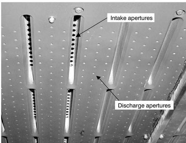
Photo 2 Appearance of nozzle panel for hot-air discharge.
