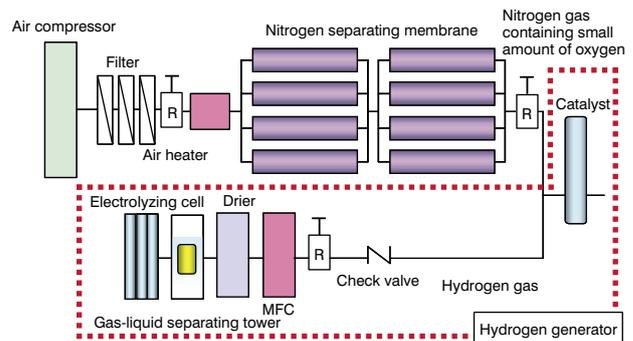
**Figure 12 Schematic of nitrogen separating system.**
