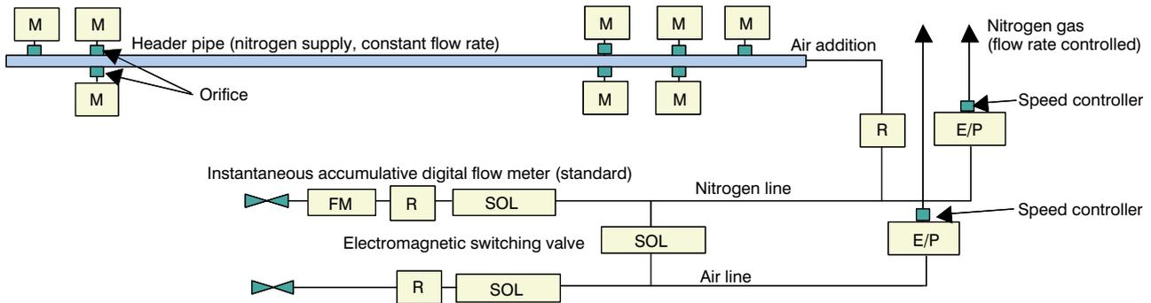
Figure 9 Nitrogen supply method.
