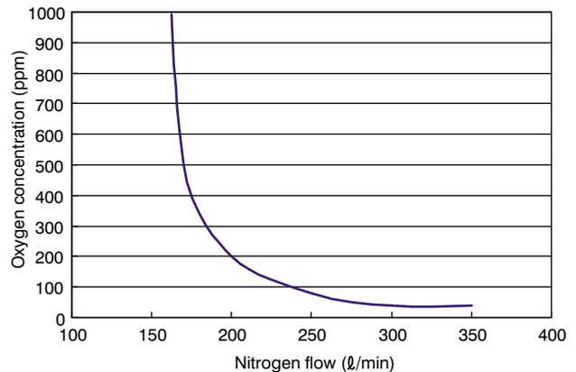
Figure 10 Relationship between oxygen concentration and amount of nitrogen supplied.
