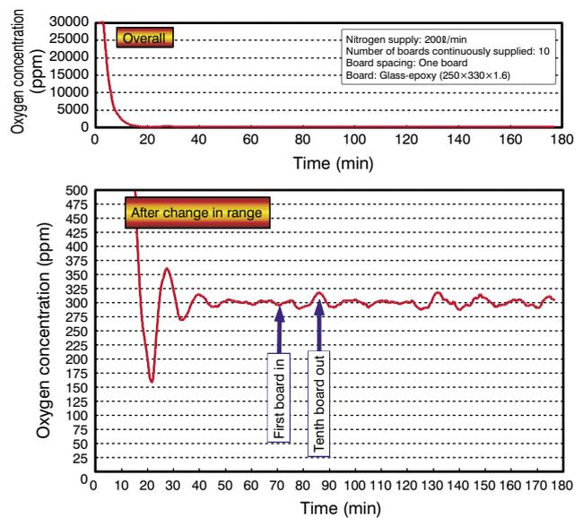
Figure 11 Stability of oxygen concentration under continuous supply.
