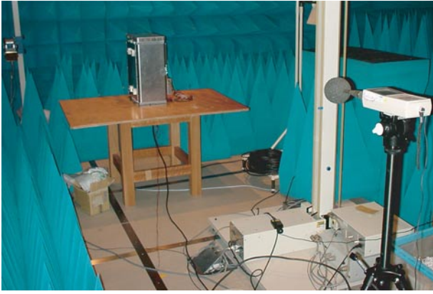
Photo 2 Experimental setup for noise measurement.
