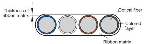
Figure 3 Structure of four-fiber ribbon.
