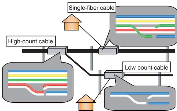
Figure 1 Cabling diagram for mid-span branching.
