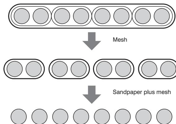
**Figure 6 Separation of separable eight-fiber ribbon.**
