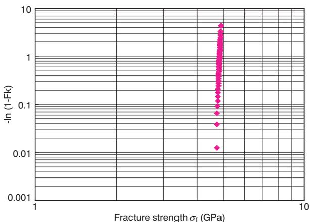
**Figure 8 Weibull distribution of fiber fracture strength after separation.**
