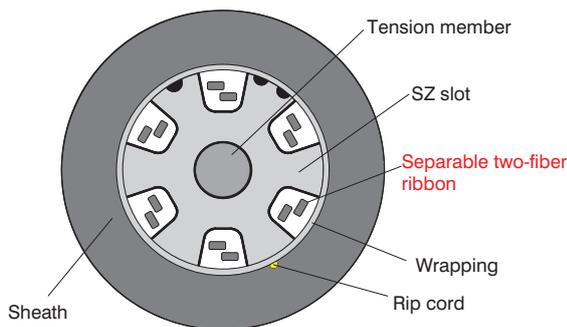
**Figure 9 Structure of SZ cable using two-fiber ribbon. (24-fiber cable)**
