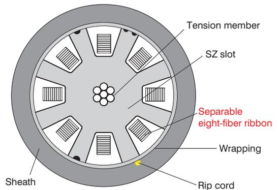
**Figure 10 Structure of 640-fiber SZ cable using eight-fiber ribbon.**
