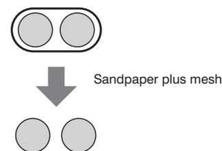
**Figure 5 Separation of separable two-fiber ribbon.**
