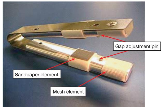
Figure 2 Fiber ribbon separation tool for mid-span branching.
