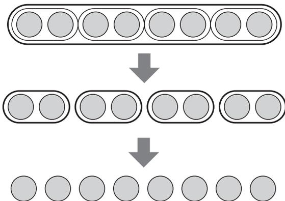
**Figure 4 Structure of separable eight-fiber ribbon.**
