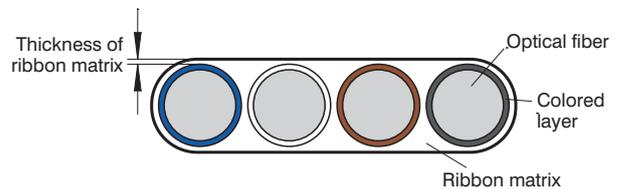
Figure 3 Structure of four-fiber ribbon.
