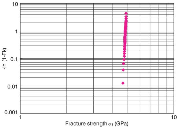
**Figure 7 Weibull distribution of fiber fracture strength before separation.**
