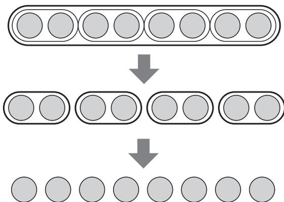
**Figure 4 Structure of separable eight-fiber ribbon.**
