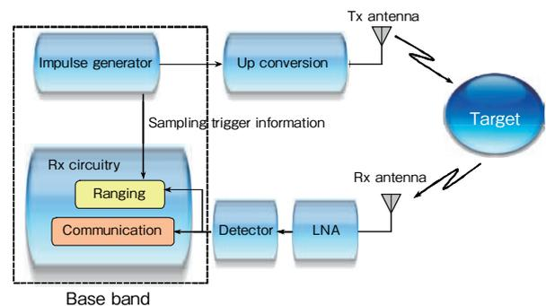
Figure 9 Schematic diagram of multi-function radar.
