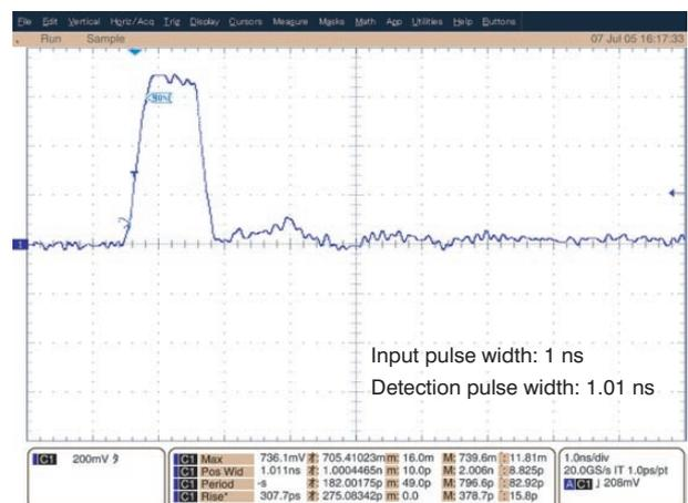
Figure 7 Typical video signal detected.
