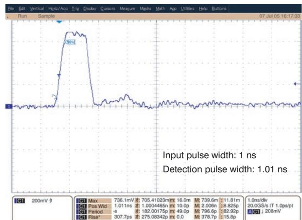
Figure 7 Typical video signal detected.
