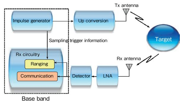
Figure 9 Schematic diagram of multi-function radar.
