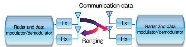
Figure 8 Block diagram of the communications and ranging device.
