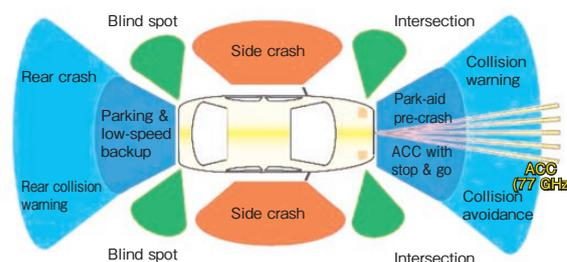
Figure 1 Possible applications for 24-GHz UWB radar.
