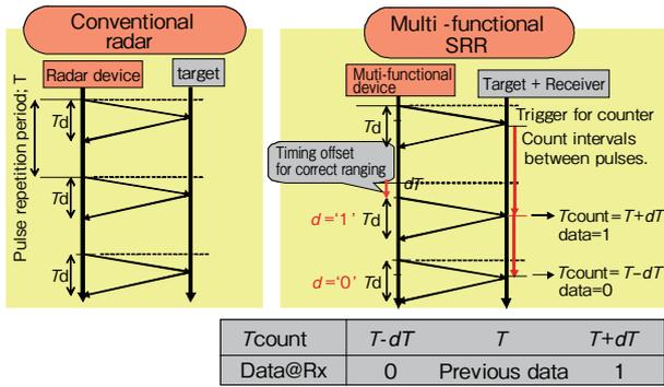
Figure 10 Flow of communication and ranging procedure.
