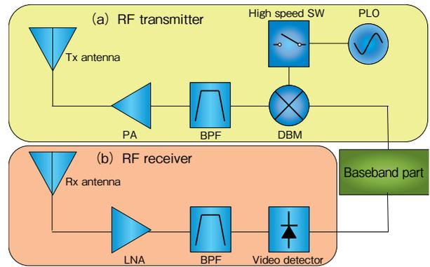
Figure 6 Schematic diagram of RF parts of radar.
