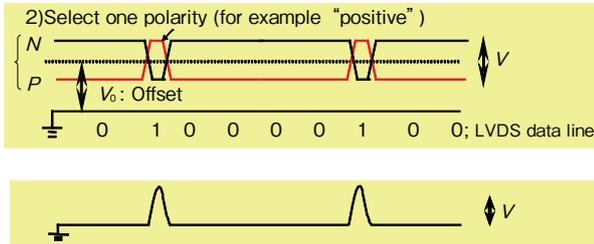
Figure 3 Impulse generated with LVDS.
