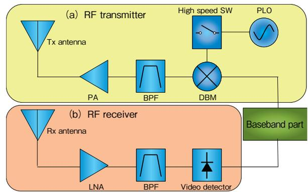
Figure 6 Schematic diagram of RF parts of radar.
