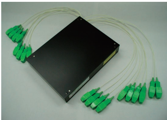
Figure 1 Appearance of high-power multiport optical amplifier for CATV.
