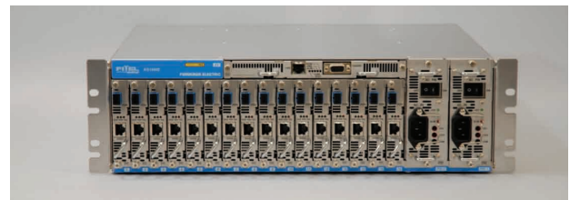
Figure 7 GE-PON central station OLT (FITELwave AG1600E).
